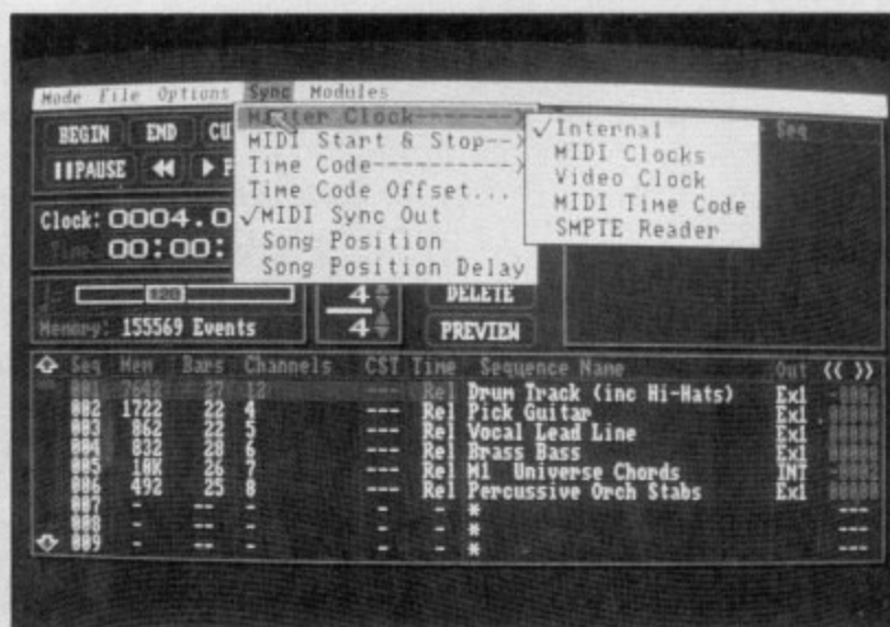
The sequencer page allows instrument parts to be recorded one by one
